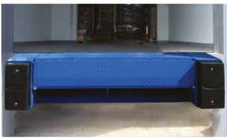
Minidock is an efficient and economical solution as it does not require power supply and can be operated manually by one person.
